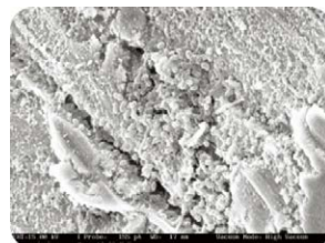
Titanium. A homogeneous layer of cocci or filamentous bacteria covers the titanium surface
